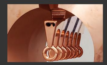
**C-band Structure -** Designed and fabricated high precision C-band Accelerator split-section structure for Los Alamos National Laboratory
